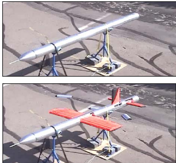
Figure 1: FASM/QuickLook UAV During Ground Testing With Integrated Ballute Module – Undeployed and Deployed Configurations
