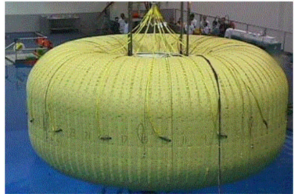
Figure 12. 30 ft Diameter Transhab Test Unit
