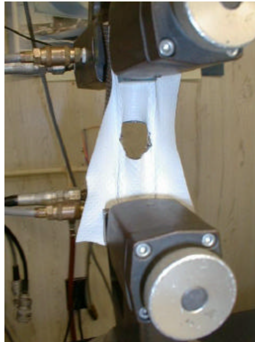
Photo 7 – Cut Slit Tear Testing In Progress
