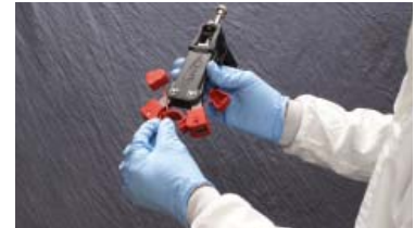
Load crimp into installation tool
