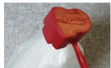
Install crimp cap on crimp body
