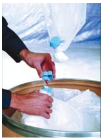
Unique Dover-Pac® crimping system is used to separate filled drum
