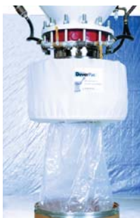
Next sleeve is pulled into drum
