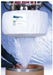
Sleeve is pulled into drum and filled
