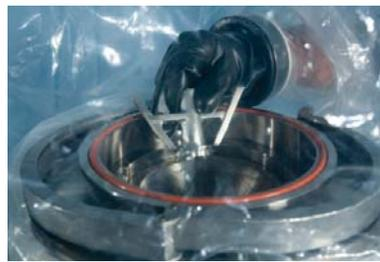
Figure 4. Integral glove sleeve for manipulating screen.
