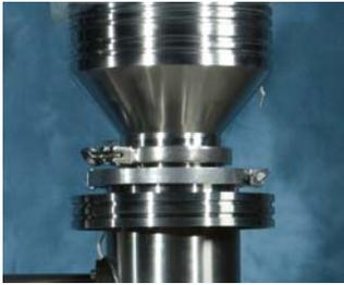
Figure 3. Grooved interface ring
