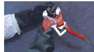
Load crimp into installation tool
