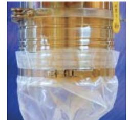
Canister and Transition Adapter Attached to ILC Dover Test Rig.
