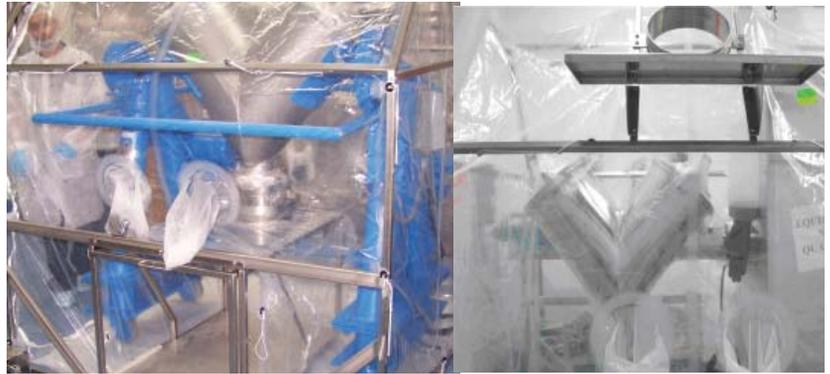
The enclosures are manufactured from clear ArmorFlex® 113 film that allows room light to illuminate inside the enclosure for easy viewing. This rugged film provides a safe working environment while enabling the enhancements developed through numerous installations using this flexible containment technology.
