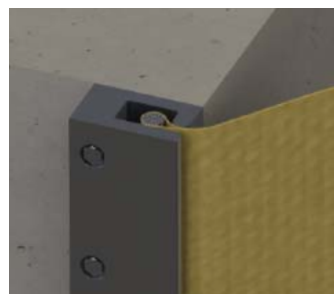
GATE GUIDE AND DEADMAN
