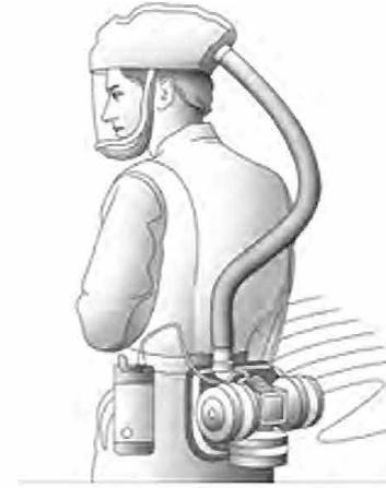
**Loose-Fitting Powered Air-Purifying Respirator (PAPR)**
