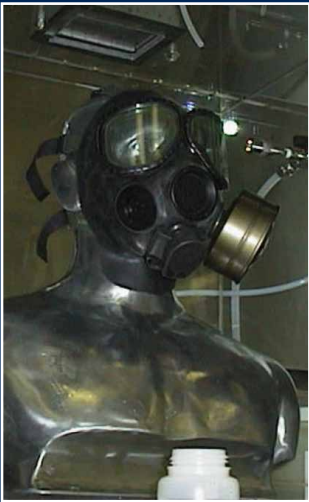
Simulant Agent Resistant Test Manikin (SMARTMAN) head form shown with M40 mask.
