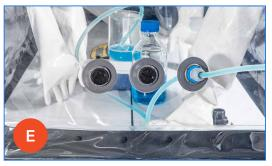
Photo of (A) a single-use isolator (soloADC from ILC Dover) for high-potency ADC payloads handling; (B & C) single-use isolator operation wearing powered air purification respirator (PAPR); (D) BIBO process using continuous liner welding; (E) pre-welded peristaltic pump hose line ports on single-use isolator
